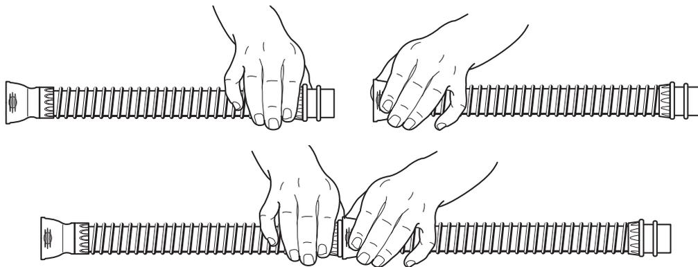
Connect the 2 ft. hose section to the Wall Adapter and the Star Control® Assembly to the opposite end of the 2 ft. hose section.
