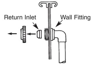
For a **1.5" Female Fitting**, thread the Zippy Wall Adapter into the wall fitting as shown.
