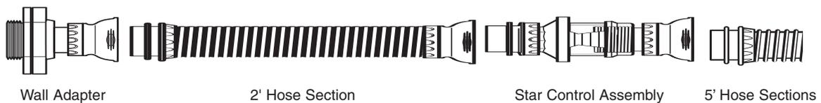
In proper order, connect the number of 5 ft. hose sections needed for your pool to the Star Control Assembly. Hose and hose floats must be assembled as shown below for Zippy to perform properly.
