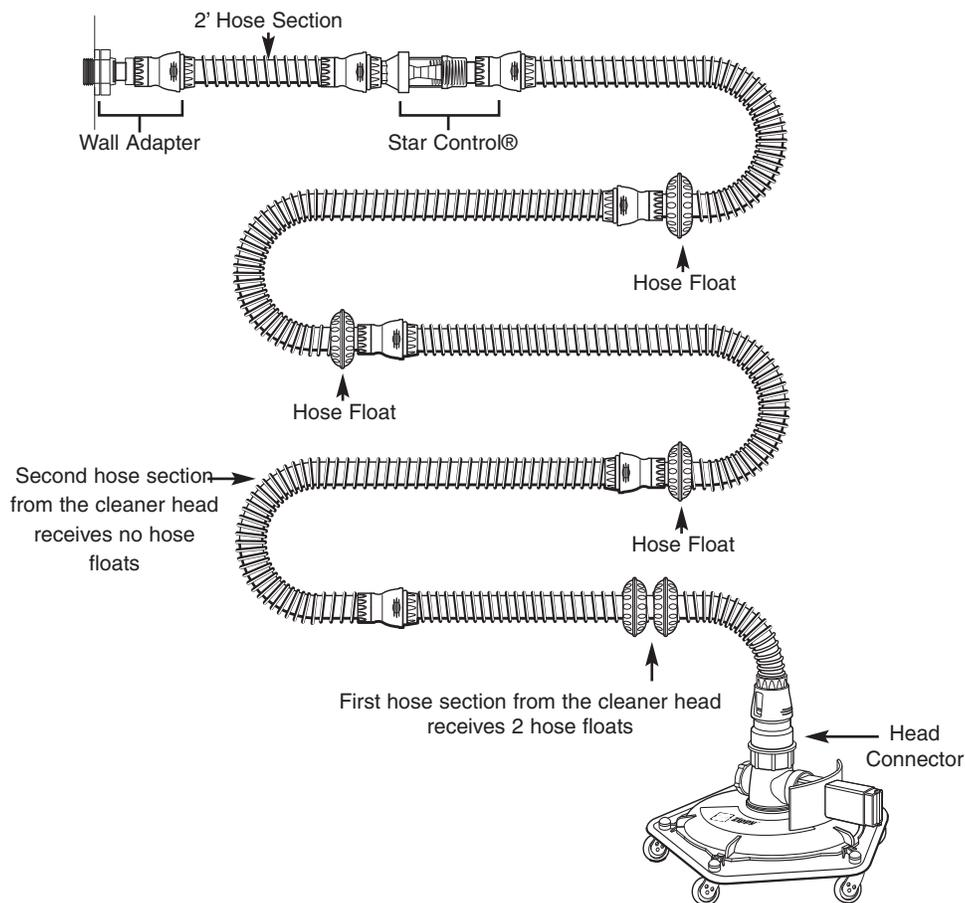
Thread the head connector that is attached to the first hose section onto the cleaner head. Submerge the Zippy head in the pool, tilt it on its side and wiggle it back and forth until the air is evacuated and bubbles cease. Then, lower the Zippy to the bottom of the pool.
